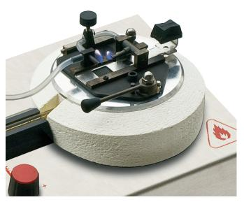
The Rapid Tester® is ideal for routine flash point testing:
