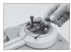
3. Introduce test flame - observe flash or no flash. Test complete.
