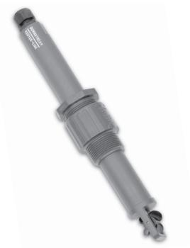
Turbo-Flo™ probes offer the precision of turbine technology with rugged construction. The practical design of the probe includes a bluff bar which protects the turbine from foreign materials in the stream as well as from over insertion. Installation is simple and does not require special fittings. The Turbo-Flo™ probe may be installed in standard pipe tees, through pipe saddles, welding spuds and 1½" full opening ball or gate valves.
