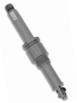
Turbo-Flo™ probes offer the precision of turbine technology with rugged construction. The practical design of the probe includes a bluff bar which protects the turbine from foreign materials in the stream as well as from over insertion. Installation is simple and does not require special fittings. The Turbo-Flo™ probe may be installed in standard pipe tees, through pipe saddles, welding spuds and 11/2" full opening ball or gate valves.
