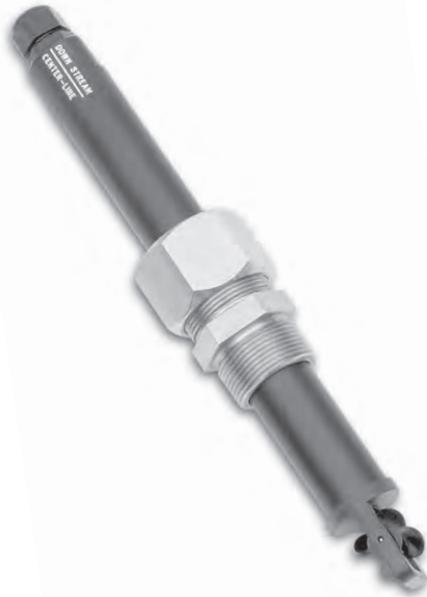
Turbo-Flo™ probes offer the precision of turbine technology with rugged construction. The practical design of the probe includes a bluff bar which protects the turbine from foreign materials in the stream as well as from over insertion. Installation is simple and does not require special fittings. The Turbo-Flo™ probe may be installed in standard pipe tees, through pipe saddles, welding spuds and 1½" full opening ball or gate valves.
