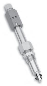
Turbo-Flo™ probes offer the precision of turbine technology with rugged construction. The practical design of the probe includes a bluff bar which protects the turbine from foreign materials in the stream as well as from over insertion. Installation is simple and does not require special fittings. The Turbo-Flo™ probe may be installed in standard pipe tees, through pipe saddles, welding spuds and 1½" full opening ball or gate valves.
