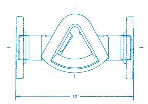
**Pressure Limits:** 200 psig (13.8 bar) with glass window 100 psig (6.8 bar) with polycarbonate window
