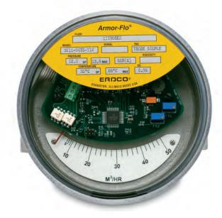
Armor-Flo™ meters with integral transmitters provide an ideal combination - a local mechanical flow rate indicator independent of electrical supply with a 4-20 mA two wire loop powered signal output. The output signal is linear within the middle 80% of the range. A response curve is furnished with each flowmeter. Simple design, rugged construction and good value make this the ideal utility fluid flowmeter.
